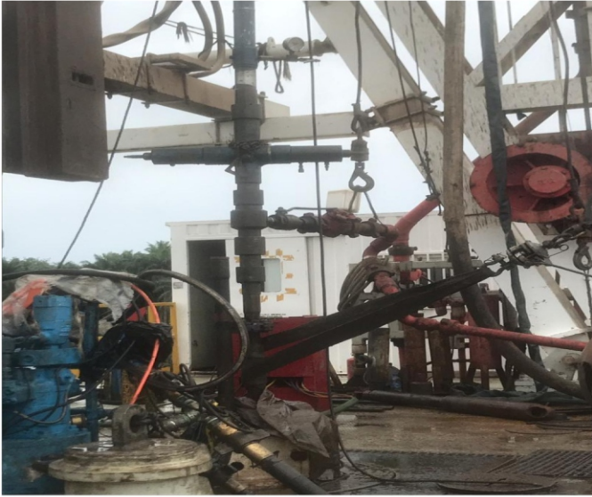
Pressure Control Rigged-Up on Tubing for Completion Operations
